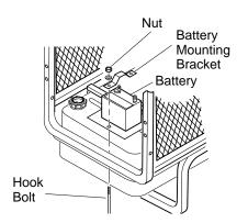
Figure 13 - Battery Hold-Down System (Model RGH11000AIE Shown)
